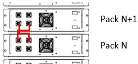
Wrong connection mode 3
